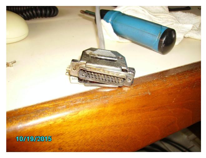
Before looking for a connector to replace this one with burned off pin at #1 I decided to check the resistance to the motors from this end of the cable. They were open on the couple I checked, and it was thought that maybe the cable was cut or blown open somewhere. All goes downhill from this point. No breaks were found in the control cable right up to the antenna. But during this inspection we did find the coax was missing about a foot of shield and its' insulation.
