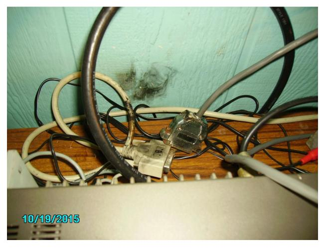
The white cable is a connector to the logic unit for the 10 position antenna switch; this logic unit was not connected to anything except another cable just like it over to the other operating position. The gray cable with the silver connector goes down to the filter box with  $6 - \frac{1}{4}$  wave stubs in it. The black cable going out to the left goes to the interface unit on the Kenwood to a USB input on the computer. Here is the USB to RS-232 interface from the Kenwood.
