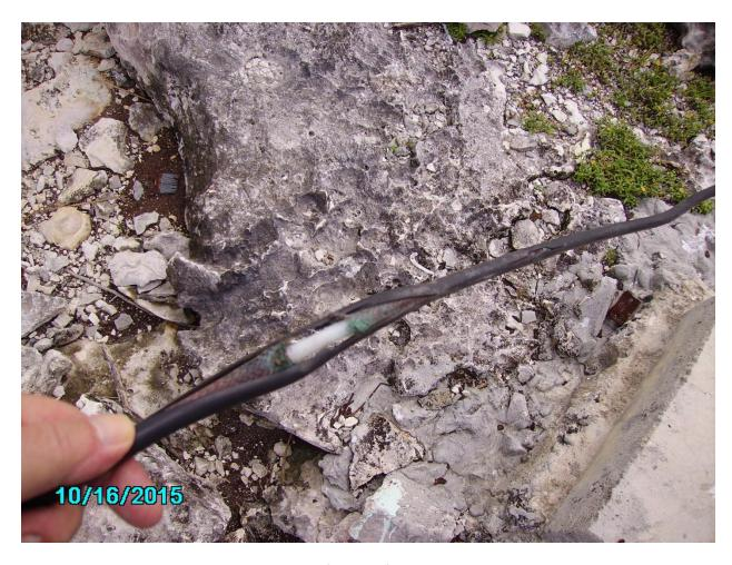
I cut back the coax towards the shack about 2 feet and found the cable to be very clean and not damaged so a new connector was installed, and another new piece made to go up to the antenna with a PL-258. When we tried to remove the PL-259 from the driven element of the antenna this happened.
