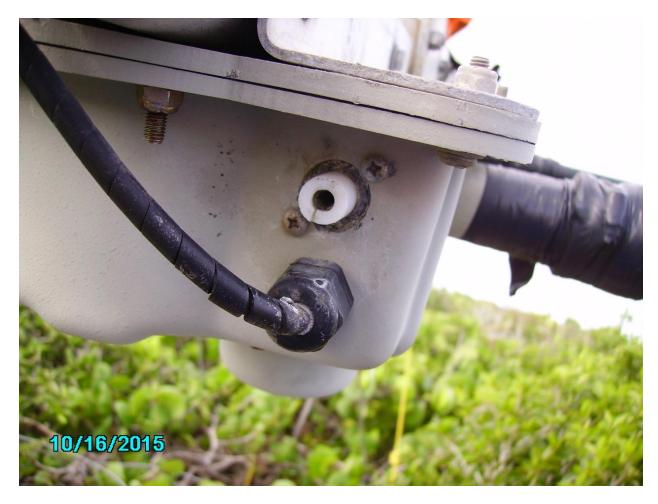
The shell of the PL-259 came off with the threads of the female completely. Well this could be fixed anyway. We took the EHU off the antenna and proceeded to put it on the picnic bench to make repairs.
