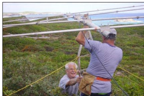
Captain Ron, N4KE and Mike N4EPD set up the 4 element 10 meter beam on a short tower section, pointing it in the ‘general direction’ of the US. Despite its low height the antenna played very well because 10m was wide open!
