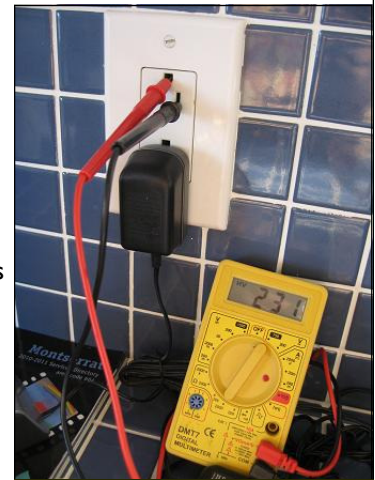
231v measured on a 110v line!
